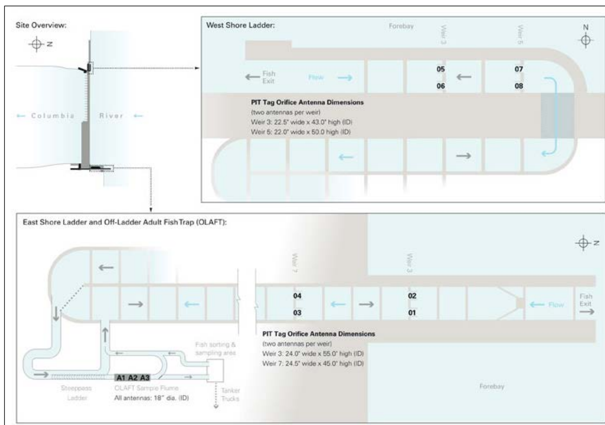
Figure 4 Plan view of upper regions of the fishway at Priest Rapids Dam showing location of PIT-tag detection antennae and associated identification number.
