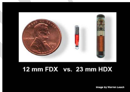
Figure 1 Relative sizes of full duplex (FDX) PIT tags as used in salmon research and the larger half duplex (HDX) PIT tags used in adult Pacific lamprey research.
