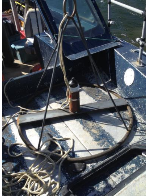
Figure 6 Metal VR2W deployment frame used in 2015 at acoustic monitoring station VRRM 413.5 and VRRM 396.1.
