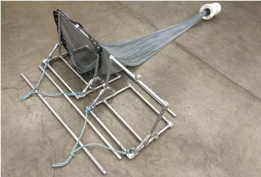
Figure 5. Modular aluminum plankton net frame. The two single frames can be reassembled into a double frame configuration by replacing three of the short horizontal members with the three long tubes.
