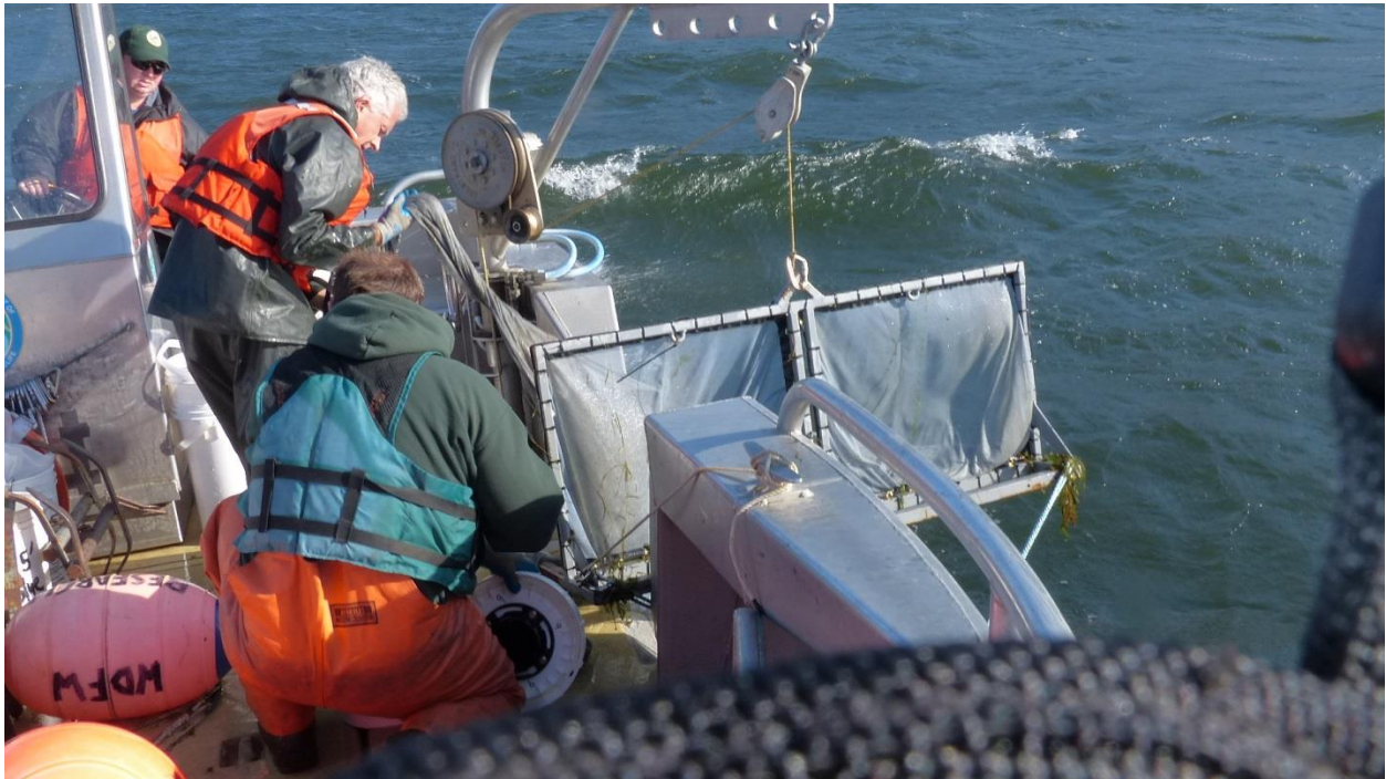
Figure 4. Photograph aboard the WDFW research vessel showing retrieval of a double plankton net frame under typical operating conditions encountered in 2015.
