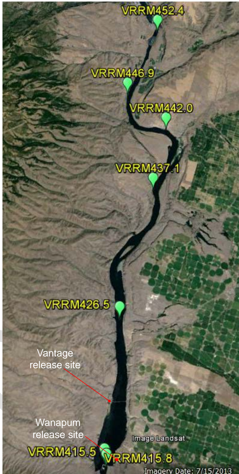
Figure 1 Locations of current Vemco VR2 acoustic receivers in Wanapum Reservoir deployed for the sturgeon monitoring program. The last four digits of each label (VRRMXXX.X represent the river mile at the deployed location.
