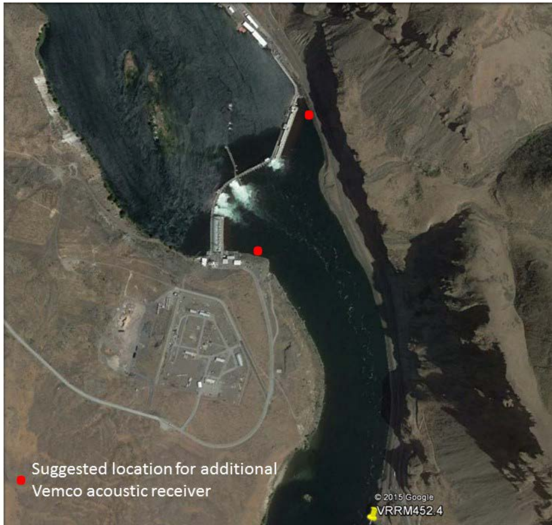
Figure 3 Proposed locations for the placement of two additional Vemco VR2 acoustic receivers in the tailrace of Rock Island Dam.
