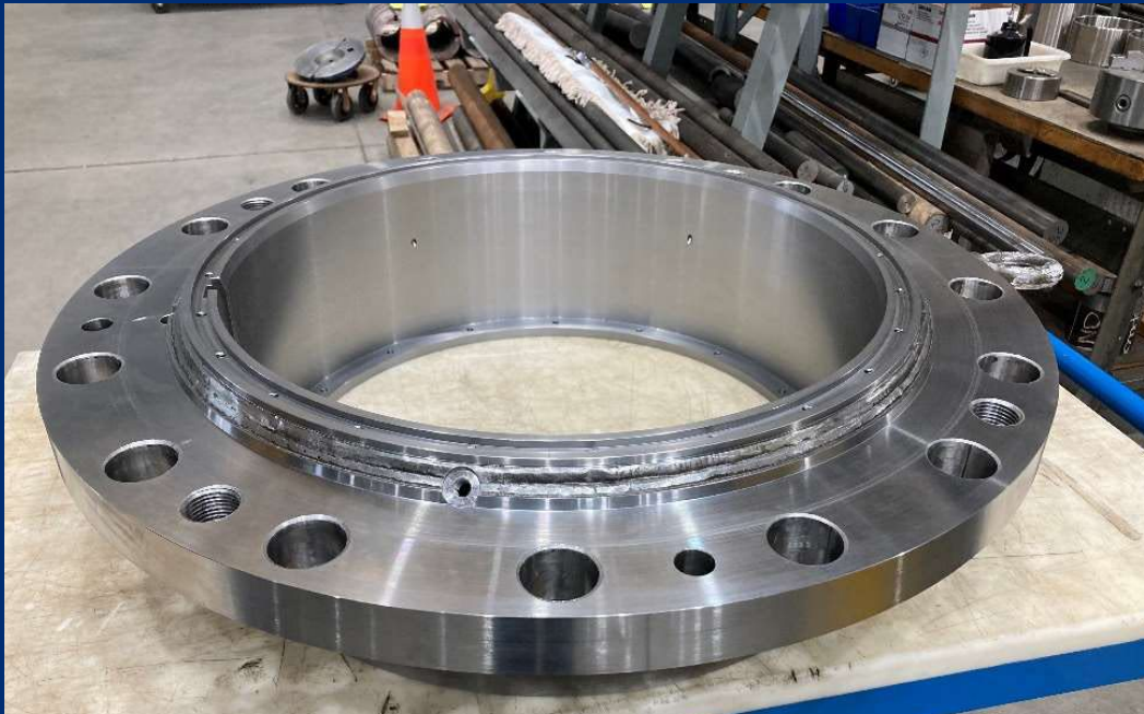
New Bearing Housing- Machined in-house
