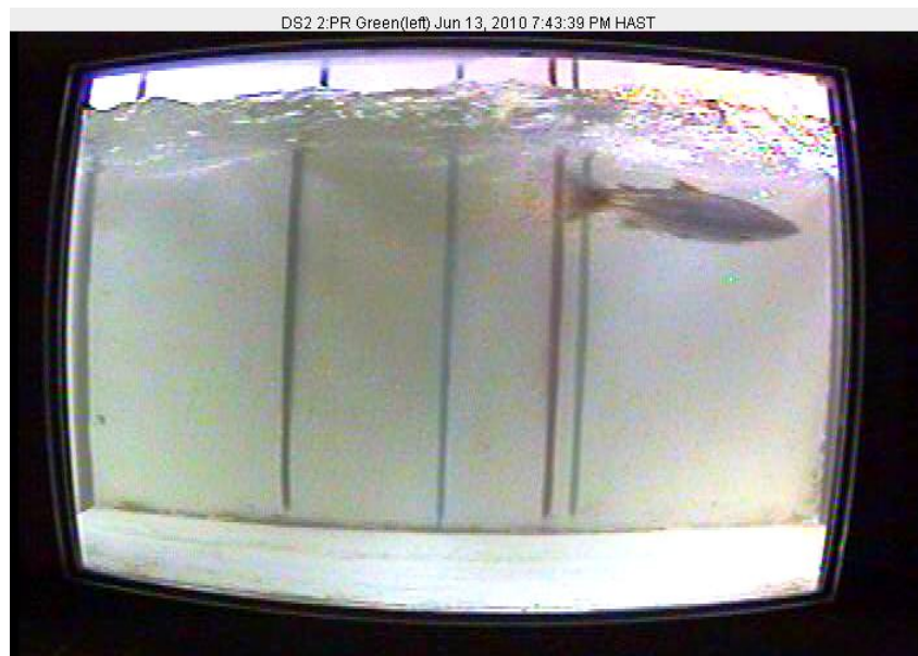
Figure 1 Bull trout passing Priest Rapids left bank count station on June 13, 2010. The blue line is 12” from the black line and the red and green lines are 20” and 22” from the black line respectively.
