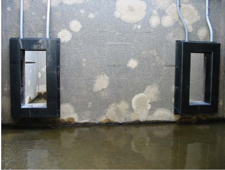
Figure 2 PIT-tag antennae mounted to the upstream face of Weir 3 in the Priest Rapids Dam east-bank adult fishway.
