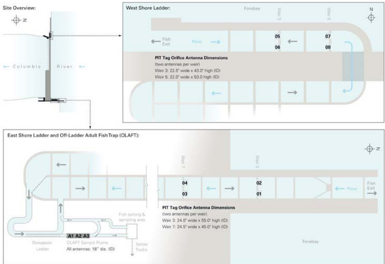
Figure 1 Plan view of upper regions of the fishways at Priest Rapids Dam showing location of PIT-tag detection antennae and associated identification numbers
