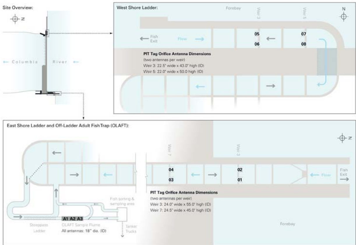
Figure 1 Plan view of upper regions of the fishways at Priest Rapids Dam showing location of PIT-tag detection weirs the OLAFT system and coil identification numbers.
