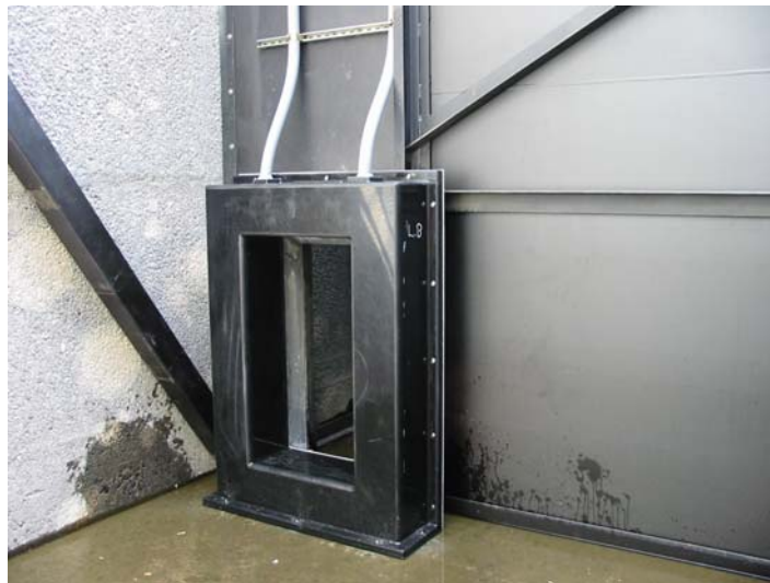
Figure 3 PIT-tag antennas mounted to the upstream side of the “video count box” of Weir 7 in the Priest Rapids Dam east-bank adult fishway.
