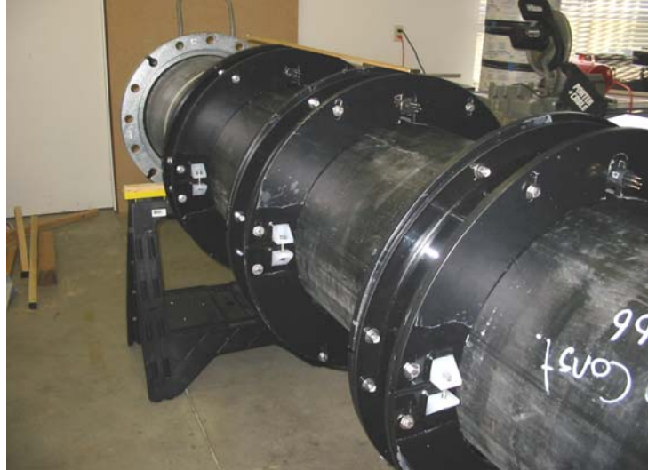
Figure 4 Picture of the OLAFT PIT-tag detection pipe with three antenna coils, prior to installation.
